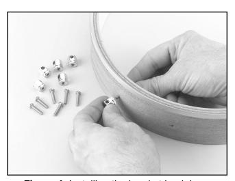
Figure 4. Installing the bracket hook lugs.
